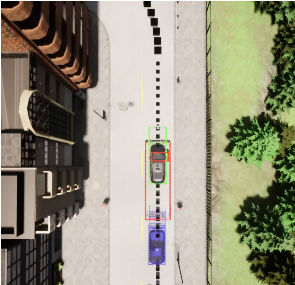
Figure 3.3: The red light detection. The small red box is the trigger box of the traffic light, colored in its state. The large red box around the car is the light detector box that follows the car. When the light detector box intersects with a red or yellow trigger box, it will turn red and the car stops.
