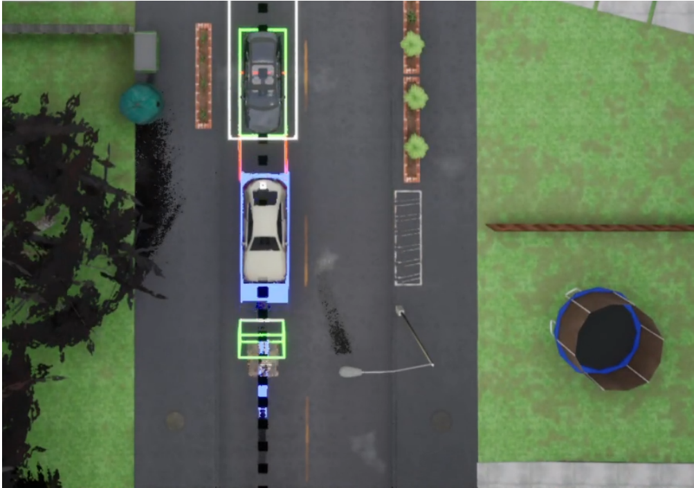
Figure 3.8: SEED keeping a safe distance to the preceding vehicle indicated by the red box.
