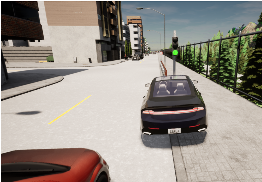
Figure 3.14: Network predicts driving straight, but the PID controller fails to execute and crashes after waiting at a traffic light.
