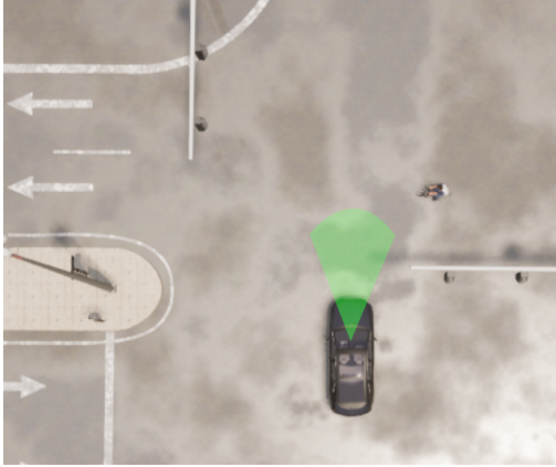
(a) False negative. No collision is predicted even though the agent is in a dangerous situation.
